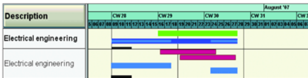
Figure 4.2 Example of Scheduling a Partially Confirmed Activity, Where the "Shift Order" Indicator Is Not Set
